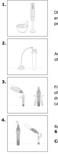
Obtain a representative sample of the specimen you want to analyze and homogenize it using a blender or a mortar and pestle. For rinse water samples, proceed to step 2.
